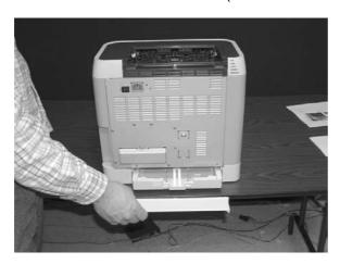
2 Remove nine (9) screws from the rear plate (RC1–5227–000CN).
