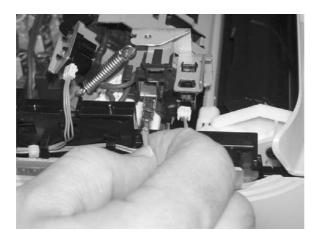
15 Remove the thermistor wire.
