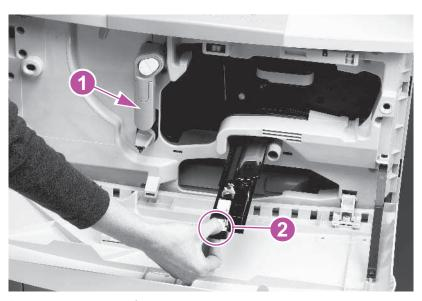
Figure 72. Removing the transfer roller assembly
