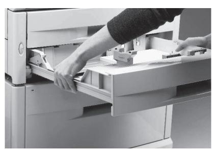
Figure 73. Removing tray 2 or tray 3
