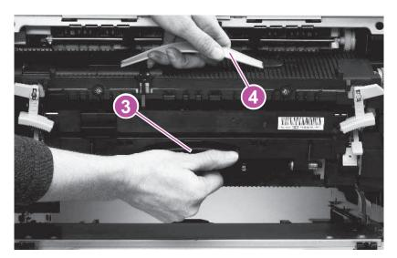
Figure 90. Removing the fuser assembly (2 of 2)
