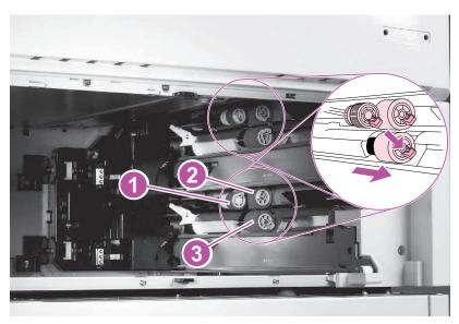
Figure 74. Removing the rollers
