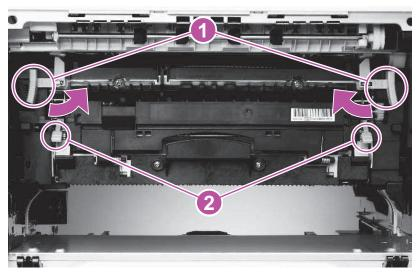
Figure 89. Removing the fuser assembly (1 of 2)
