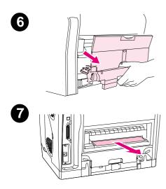
**6** Grasp the fuser handles and pull to remove the fuser from the printer.
