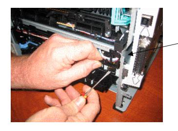
Remove Harness guide by lifting the black tab, and sliding it to the left.
