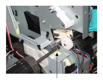
Remove left side fuser screw ( was behind the gear that you just removed).
