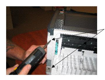
Remove screws from top & bottom of left side of fuser cover.
