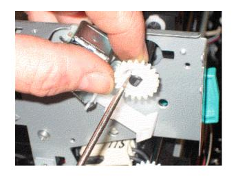
Move tab away from shaft then slide gear off shaft.
