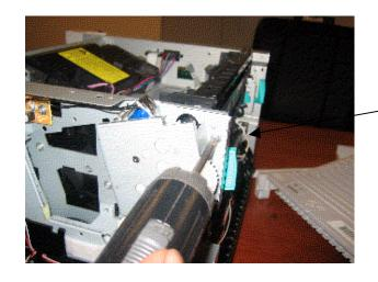
Remove right side screw from fuser drive assy.
