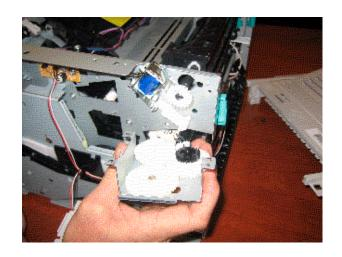
Be careful not to drop gears out of housing. Set face up on table.
