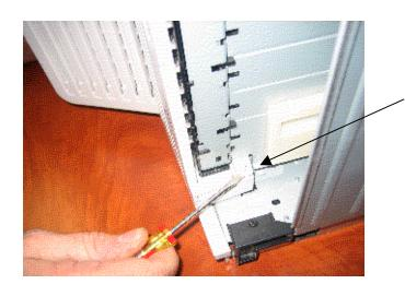
Move lock tab from pin and move rear cover away from machine.
