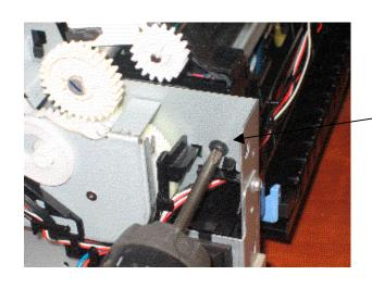
Remove fuser screw lower left side.
