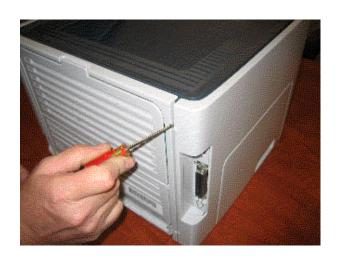
From Rear of machine, remove left cover by popping open cover from top and bottom.
