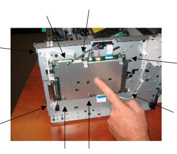
Unplug all the cable harnesses from the formatter board, then remove all the screws.
