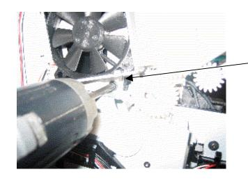
Remove fan housing lower screw.
