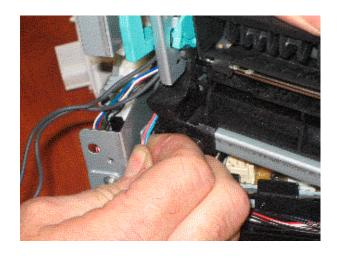
Thread left side cables from harness guide on left side of fuser, and work fuser completely out.
