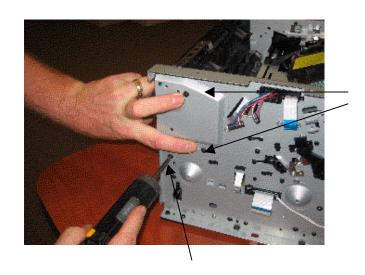
Remove right side screws from fuser.
