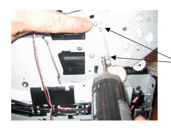
Remove gear drive left side screws.
