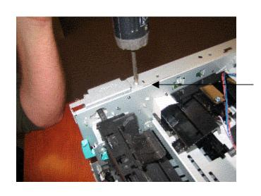
Remove screw from left rear top fuser cover drive cover.
