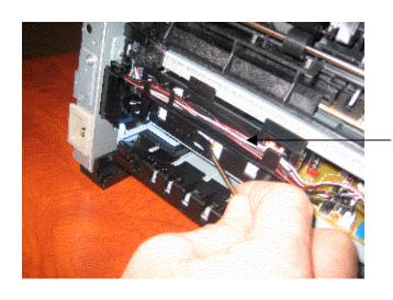
Lift tab on left side harness guide and move guide to right.
