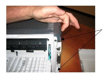
Remove screws from top & bottom of right side of fuser cover.
