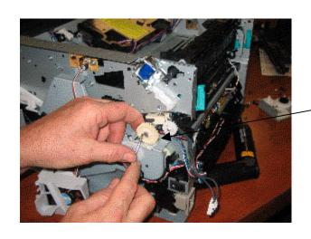
Remove left side fuser gear.
