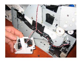
Remove fan and housing, set off to the side.
