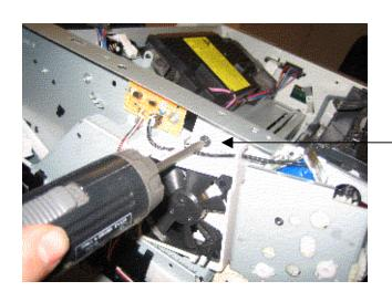
Remove fan housing top screw.
