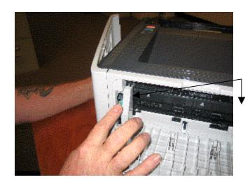
Move down both left and right pressure roller levers.
